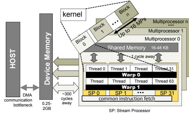
Figure 3: NVIDIA CUDA architecture.
